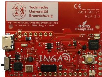
Figure 4: The INGA sensor node used in the Evaluation to prototype ClimbNet
